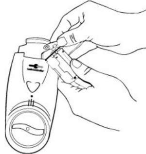
Gently disconnect the battery holder from the snap connector. Insert the 4 batteries into the battery holder slots, matching the positive (+) and negative (-) terminals. Gently reconnect the snap connector to the battery holder and insert the battery holder into the battery compartment and close the battery door.
