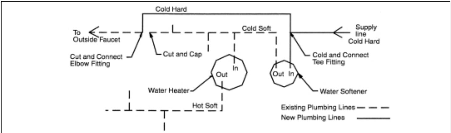
4. Attach the bypass valve to the control valve. Connect the inlet and outlet of the Iron softener to the plumbing in the house. The control valve must not be subjected to temperatures above 71°C (160°F). To avoid damaging the control valve when sweat fittings are used, solder the threaded copper adapters to the copper pipe and then, using teflon tape, screw the assembly into the bypass valve.
