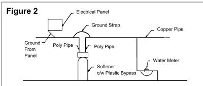
In all cases where metal pipe was originally used and is later interrupted by poly pipe or the Noryl bypass valve as in Figure 2 or by physical separation as in Figure 3, an approved ground clamp with no less than #6 copper conductor must be used for continuity, to maintain proper metallic pipe bonding.
