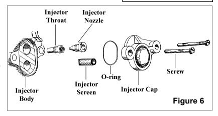
The injector orifice is removed from the injector body by carefully turning it out with a screwdriver. Remove the injector throat the same way. Carefully flush all parts with water. Use a mild acid such as vinegar or Pro-Rust Out to clean the small holes in the orifice and throat. Reassemble using the reverse procedure. Do not over tighten.
