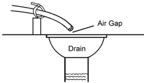
**NOTE:** Waste connections or drain outlet shall be designed and constructed to provide for connection to the sanitary waste system through an air-gap of 2 pipe diameters or 1 inch (22 mm) whichever is larger.
