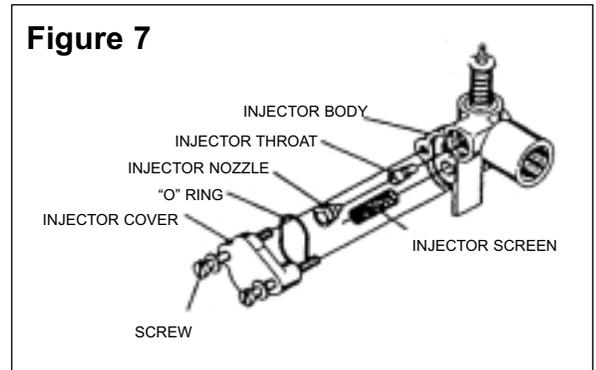
Reassemble using the reverse procedure.
