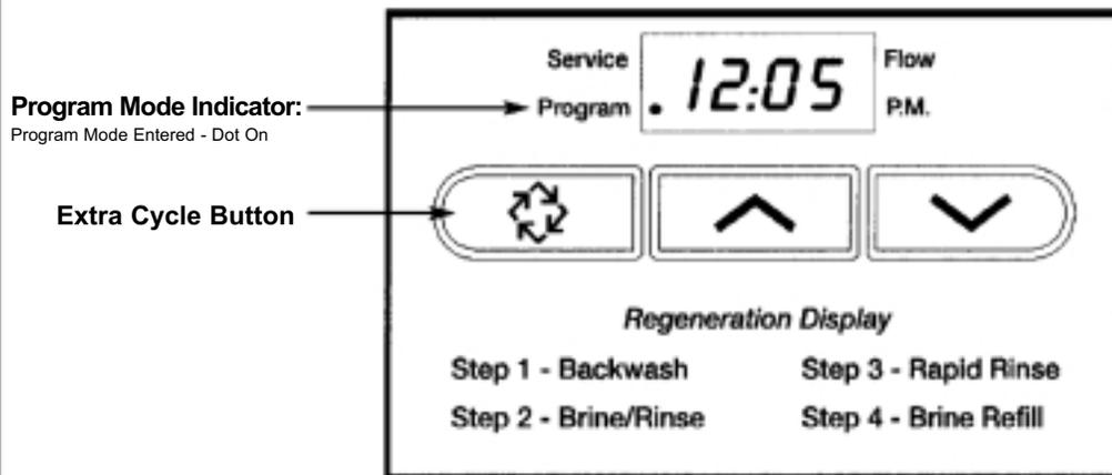
1. Push and hold for 5 seconds *both* the Up and Down Set Buttons to enter Programming Mode.
