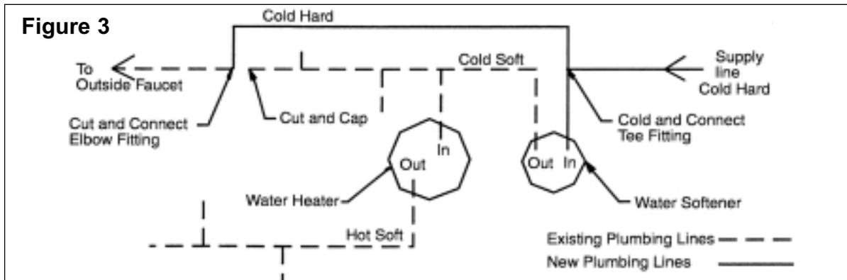
4. Attach the bypass valve to the control valve. Connect the inlet and outlet of the water softener to the plumbing in the house. The control valve must not be submitted to temperatures above 71°C (110°F). When sweat fittings are used, to avoid damaging the control valve, solder the threaded copper adapters to the copper pipe and then, using Teflon tape, screw the assembly into the bypass valve.
