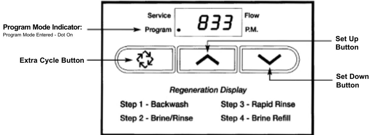
1. The first option setting display that appears in the Program Mode is Treated Water Capacity. Using the Set Up or Down Buttons, set the amount of treated water that can flow through the unit before a regeneration is required. For Example:
